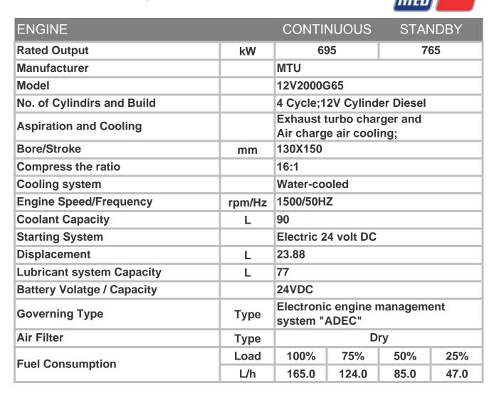
**ENGINE**--Industrial 4 stroke cooled diesel engine complete with air,fuel and oil filters,electric starting and charging equipment,engine protection against low water level.
