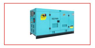
Altitude: Derate 2.0% per 300m(984 ft.)elevation above 1000m(3279ft.) up to a maximum elevation of 2450m(8000 ft.). More than 2450m(8000ft), please contacts with us or our dealer seek the help. Temperature: Derate 6.0% per 11 °C(20°F) temperature above 40°C(104°F).
