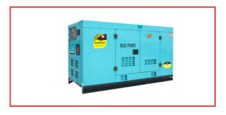
Altitude: Derate 2.0% per 300m(984 ft.) elevation above 1000m(3279 ft.) up to a maximum elevation of 2450m(8000 ft.). More than 2450m(8000ft), please contacts with us or our dealer seek the help. Temperature: Derate 6.0% per 11 °C(20°F) temperature above 40°C(104°F).
